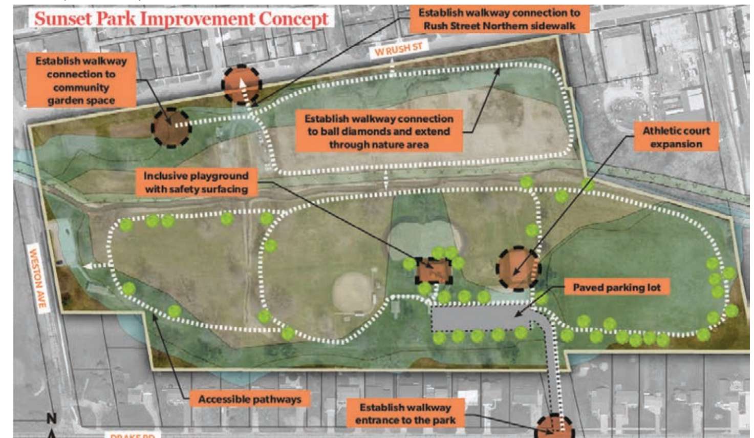
This concept drawing from the 2025-2030 Park Master Plan shows integration of walkway connections through natural areas.
